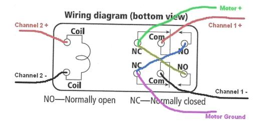
I hooked the wall warts up to LOR. Channel 1 was the 12 vdc coil and channel 2 was the 5vdc. Whenever the 5vdc was applied his head would turn left but when not applied would revert to the right.
